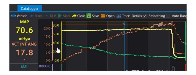
3. Right click on the axis to be adjusted and select the <u>Adjust Range</u> option. A new window will open that allows direct entry of the desired min/max display range on the chart.
