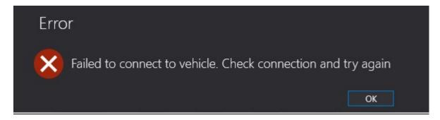
When there is no data from the PCM being received by the cable, you may receive an ERR\_BUFFER\_EMPTY or ERR\_INVALID\_DEVICE\_ID error message. In this case, unplug the J2534 cable from the PCM and laptop and then replug in the cables.
