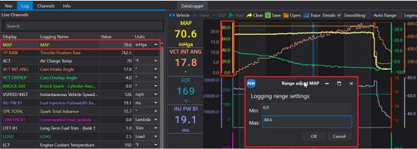
2. Hover the mouse over the axis and use the mouse scroll button, it is also possible to adjust offset by left clicking the mouse and dragging up / down,
