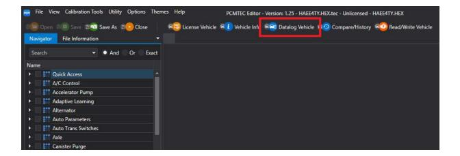
Once the Datalogger window is opened, and the vehicle ignition turned on, the data logger will automatically connect to the vehicles PCM and a set of default channels will automatically be selected.
