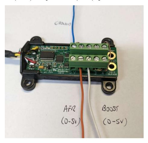
Next plug in your DLP device into your PC. It should install FTDI drivers automatically, and add a COM port to Device Manager when plugged in.
